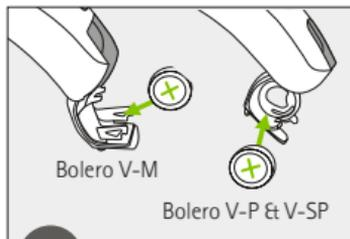
Place battery in the battery door with the "+" symbol facing upwards.
